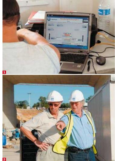
A screen at the control center displays all the movement measurements recorded by the Advitam laser telemetry sight systems.
