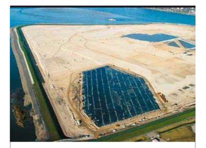
2001 In Hamburg (Germany), the Airbus A380 assembly site is built on 140 ha of land reclaimed from a dead branch of the Elbe consisting of muddy deposits. To isolate the northern zone where the work had to start in emergency, Ménard used atmospheric consolidation to create a 135,000 m<sup>2</sup> dike to a height of + 9 (8.50 m above mud level).
