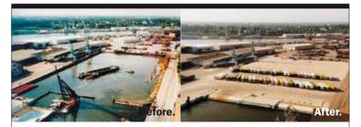
**1994** In the port of Lübeck (Germany), on the Baltic Sea, a dock unusable by modern ships was reclaimed using contaminated dredged spoils and transformed into a platform for container storage. 12 m of the platform were con-
